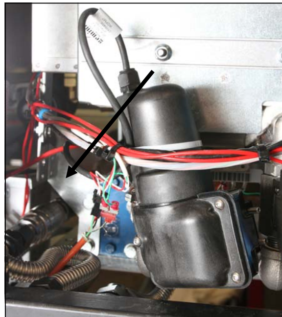
Figure 2: The actuator is shown loosened. The vertical brace (arrow) must be removed.
