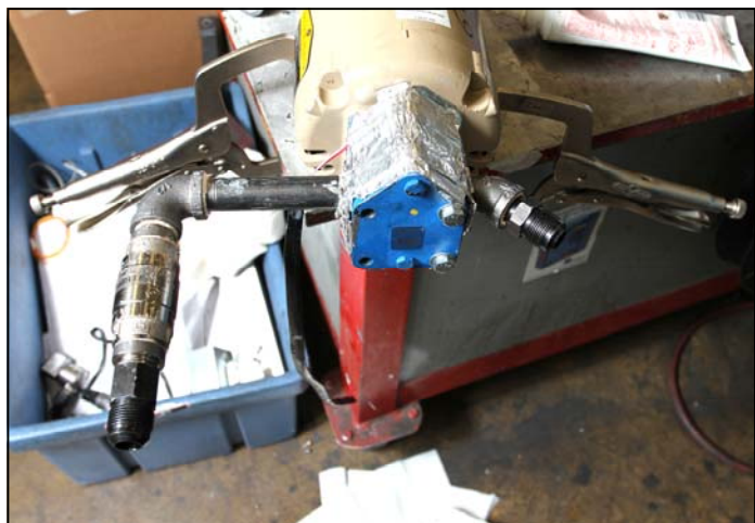
Figure 4: Reposition the check valve and elbow on the pump as shown above and in Figure 1.
