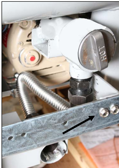
Figure 6: The pre-filter is shown in position above the filter pan. It's secured by two sheet metal screws (arrow). A flex line (shown) connects the pre-filter to the filter pan pickup. A second flex line from the side of the pre-filter leads to the lower connection on the oil quality sensor
